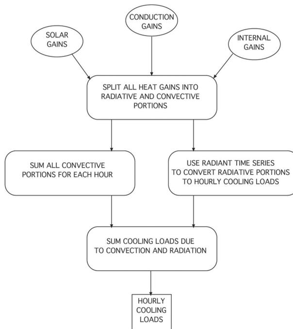
**Figure 1.2 Schematic of the radiant time series method.**
